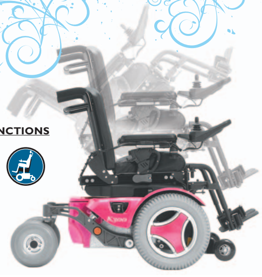
Power seat elevator and power tilt
