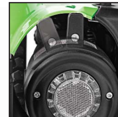
Brake release on individual motors allows the chair to be maneuvered manually
