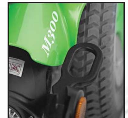
Two front and rear tie-downs for safe transport
