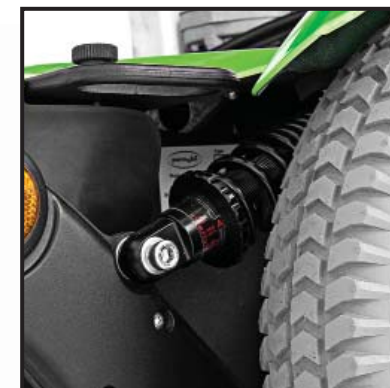
Easily adjustable suspension allows the ride to be customized to the user's needs
